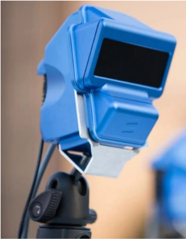
Baraja's "head" unit, connected by fiber optic to the brain.
