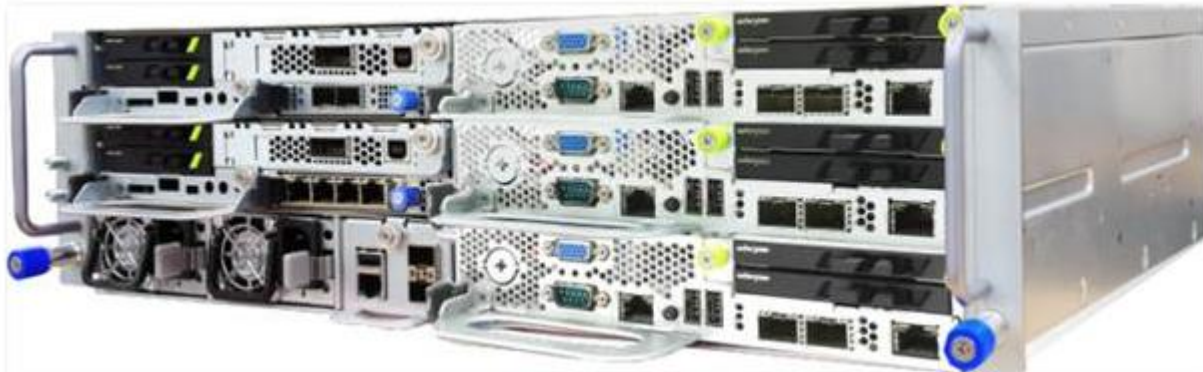
Figure 7. The openEDGE chassis design is based on Open Compute Project standards. Its shallow form factor, low power requirements, and processing density are optimized for telco and edge applications
