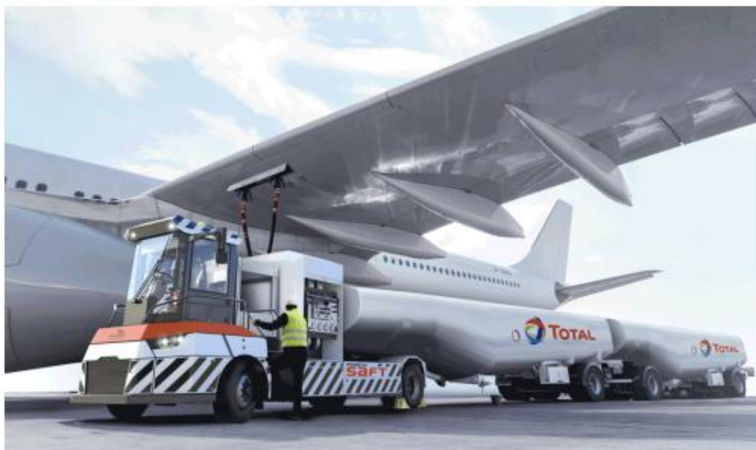
Electric Aircraft Refueler Transporter, equipped with two 30-ton fuel tanks (artist rendering – courtesy of Gaussin)
